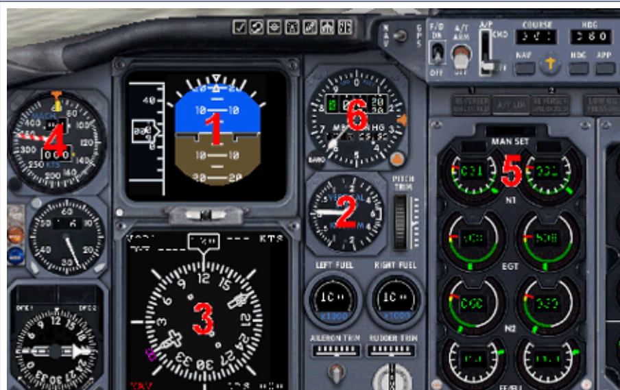
Instruments to scan: 1-ADI; 2-VSI; 3-HSI; 4-Airspeed indicator; 5-N1 percent; 6-Altimeter
